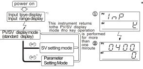
\*1 Input type and input range display When instrument is powered on, it immediately confirms the input type and input range
