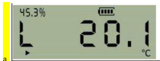
a Display the minimum temperature value and minimum humidity value of the stored data.
