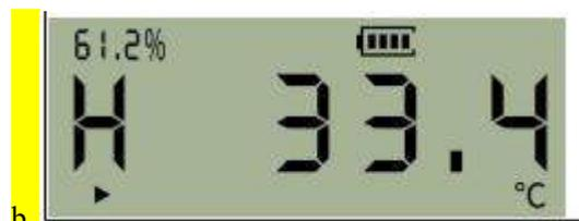
b Display the maximum temperature value and maximum humidity value of the stored data.
