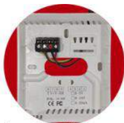
0~5V/0~10V type electrical connection diagram
