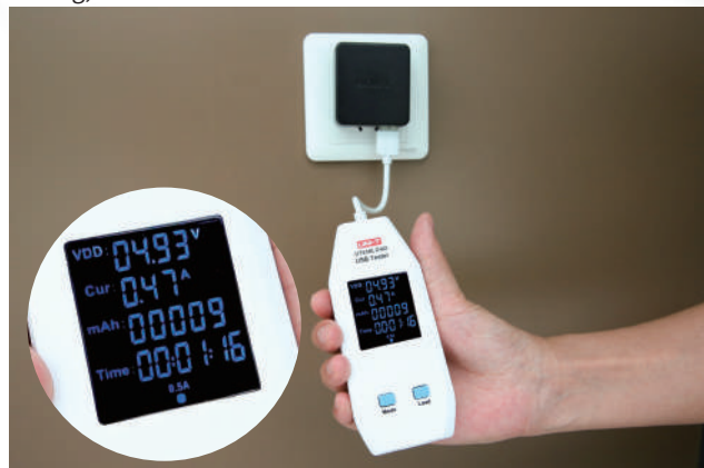
Tester with electronic load (UT658 LOAD)
