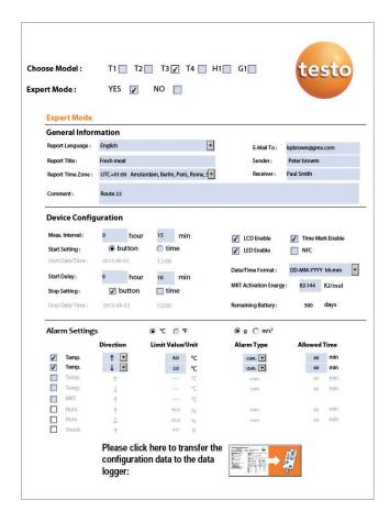
No software needs to be installed on a PC or notebook in order to configure a testo 184 data logger. The PDF configuration tool is stored on the logger itself and can be opened with a simple double-click.
