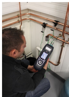
DHW network temperature
