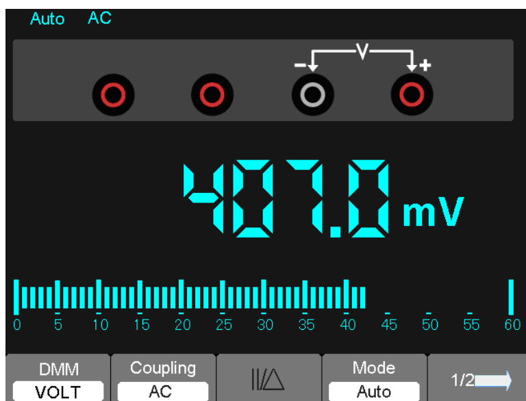
Figure 7-7 AC voltage Measurement
