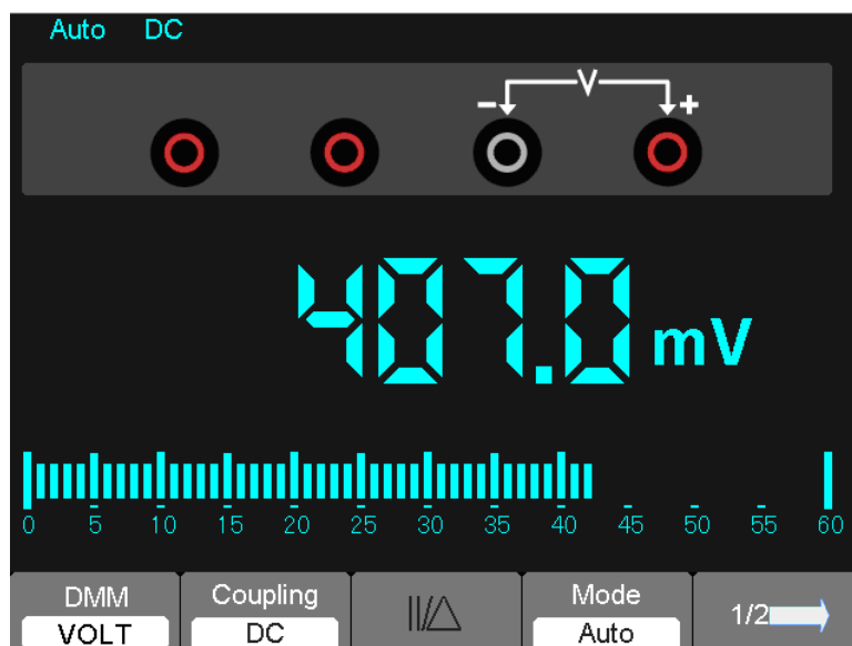
Figure 7-6 DC voltage Measurement
