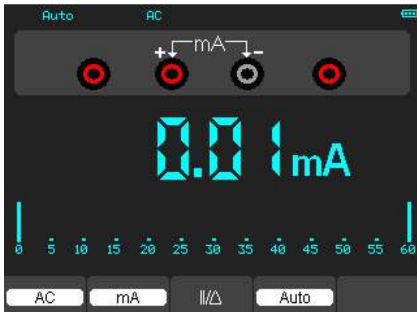
Figure 4-10 AC Current Measurement for 600 mA
