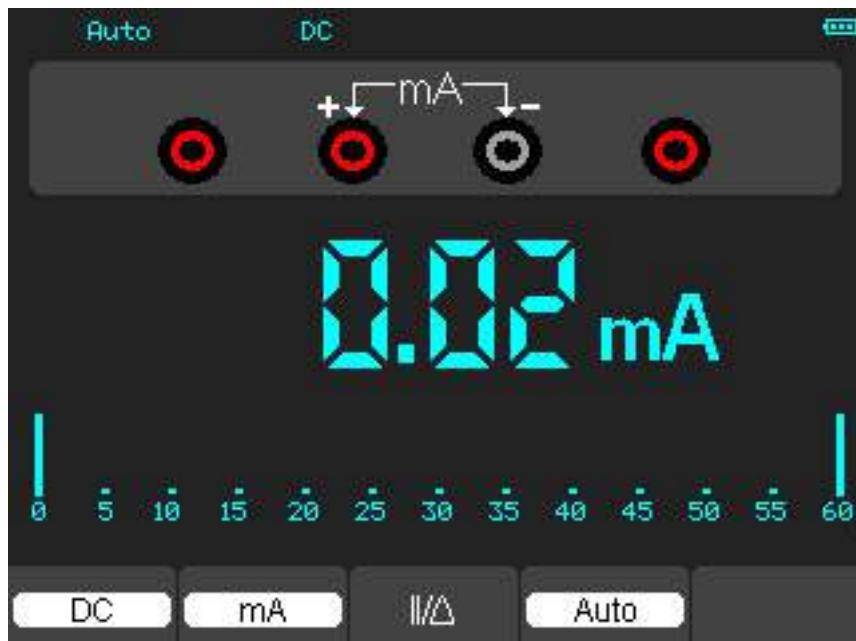
Figure 4-8 DC current Measurement for 600 mA
