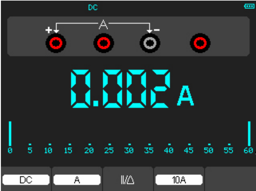
Figure 4-9 DC Current Measurement for 10A
