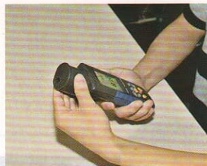
The top of 9501 can be rotated and easily used for \alpha , \beta , \gamma and X rays selection
