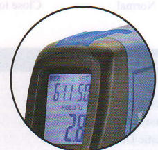
Lower temperature Located with blue LED indicator
