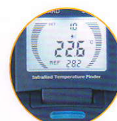
Lower temperature Located with blue LED indicator
