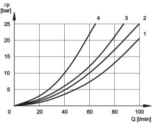
4 - PRESSURE DROPS △p-Q (values obtained with viscosity 36 cSt at 50 °C)
