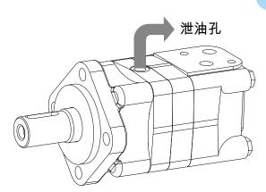
If the motor appears unsteady during low-speed operation, adding the backpressure, which is no less than 0.2 Mpa, can solve it.
