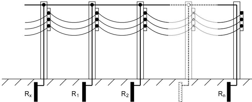
Of these earth resistances,  $R_1, R_2, \dots, R_n$  can be considered that they are connected in parallel.
